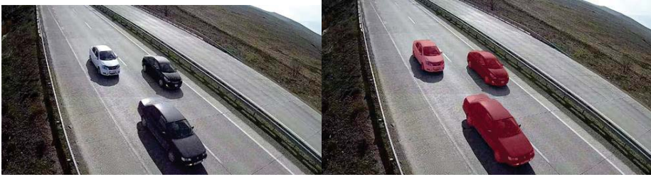
Figure 1. Example of semantic segmentation overlay using the Mask R-CNN model.
